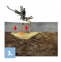
Once the void is filled, the polyurethane begins to exert upward force to lift the slab back to level.
