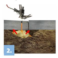
Polyurethane begins to expand and pack the void until the support is reestablished into the soil.
